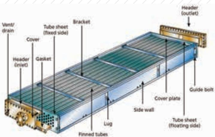
A finned tube bundle consists of finned tubes (in special cases unfinned tubes are also possible), the headers for distributing the product and a supporting frame.
