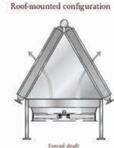
Air cooled heat exchangers in A-frame configuration are used when the plot area is restricted. The fans are arranged in forced draught.
