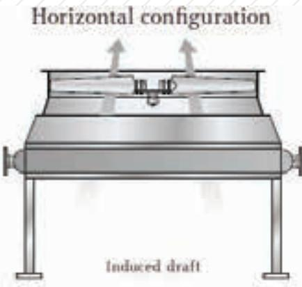
Induced draught arrangement of the fans above the heat exchanger bundles results in an even distribution of the cooling air to the heat exchanger surface. The plenum shades the heat exchanger surface and therefore protects it from solar radiation.
