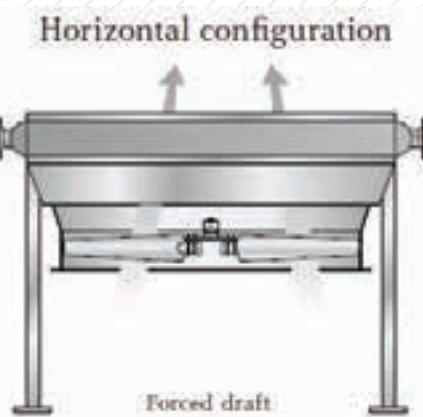
The horizontal arrangement of the heat exchanger bundles with forced draught fans underneath the bundles is the most common configuration of air cooled heat exchangers. It gives easy access to the fans and fan drives for maintenance purposes.
